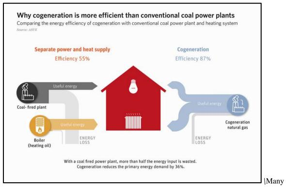
industrial and energy-generation processes produce large amounts of heat waste that is absorbed into the atmosphere.
