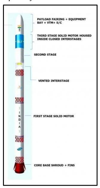
ISRO's SSLV, a small satellite launcher with big prospects ahead
